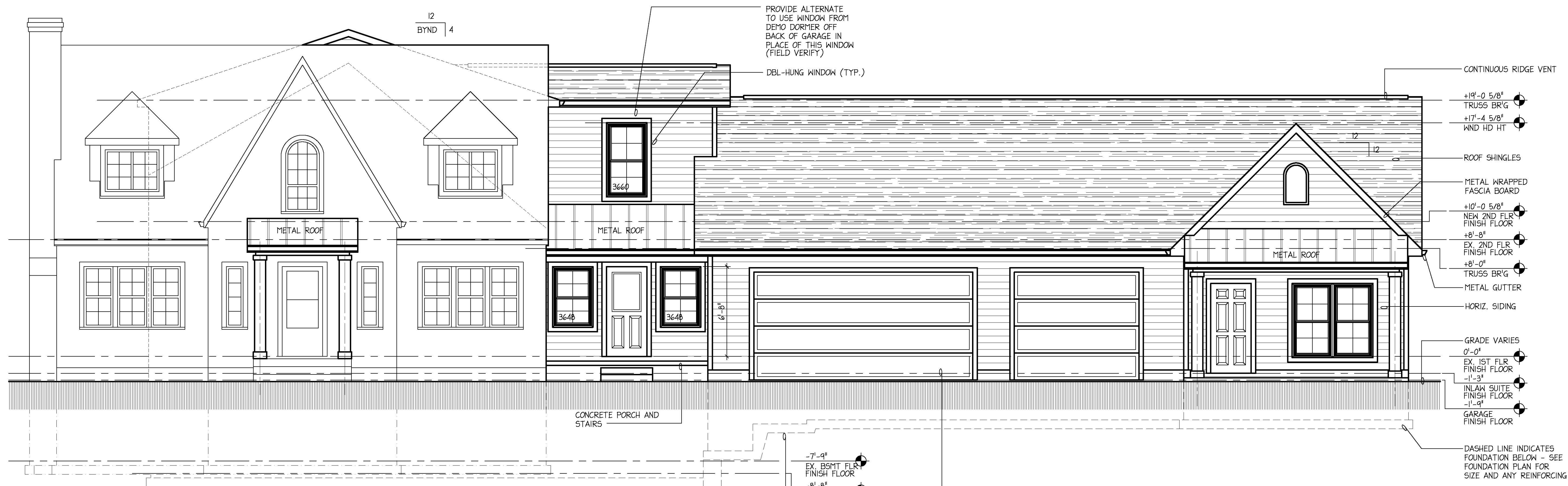
A EXTERIOR 'FRONT' ELEVATION SCALE: 1/4"=1'-0"
